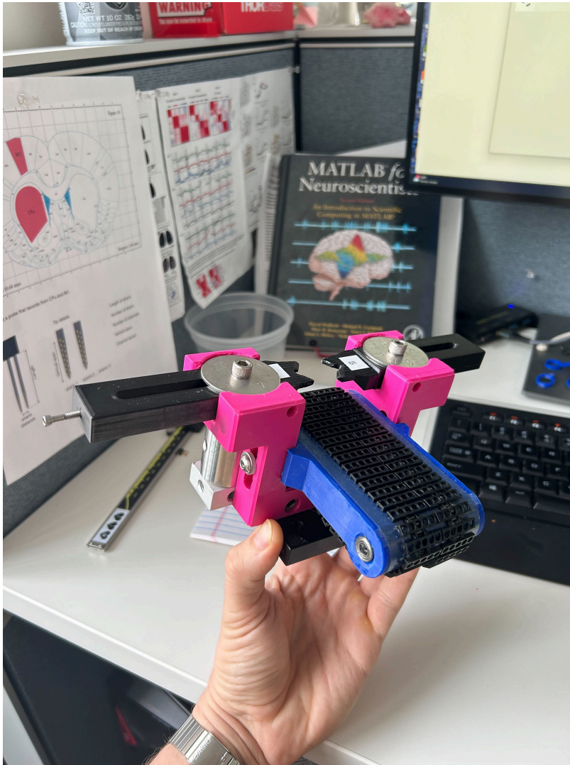
Figure 3: The finished, low-profile treadmill build — belt-driven, rotary-encoded, and sized to keep the mouse close to the pivot point so goniometer tilt corrections no longer translate into large lateral shifts.
